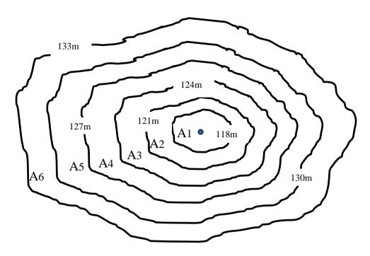
b) – Design Engineers have a proposal for construct a dam to raise a water store level up to 140m with 4m of free board and it can cover 22 hectare of catchment area at 136m level. What is the maximum safe water capacity can store in the reservoir according to the new proposal?
