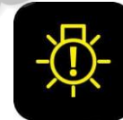
Exterior Light Fault
