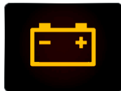
Charge warning light
