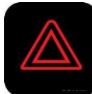
Hazard Lights on
